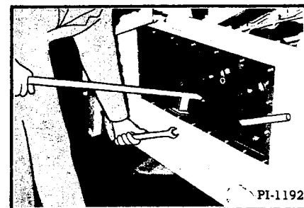
Fig. 99 Tightening Final Drive Chains
