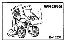
Disconnecting or loosening any hydraulic tubeline, hose, fitting, component or a part failure can cause lift arms to drop. Do not go under lift arms when raised unless supported by an approved lift arm support device. Replace if damaged.
