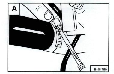
Remove the solenoid from the recovery tank bracket [B].
