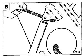
Remove the clip at the lower pivot pin C.
