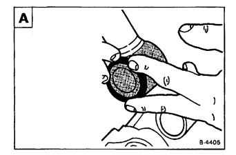
Put a piece of shim stock on each side of the seals B.
