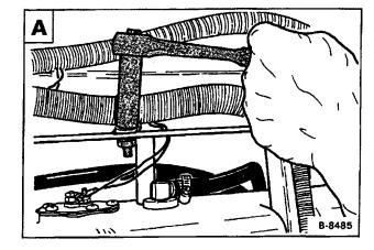
Disconnect the fuel return hose at the tank B.
