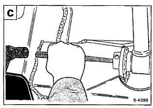
Loosen the bolt at the Bob-Tach pivot pin lacksquare. DO NOT remove the bolt.
