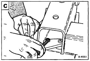
Using a punch and hammer, remove the Bob-Tach wedge and spring assembly from the frame  ${\bf D}$  .
