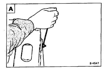
Hit the bolt to start the pivot pin into the Bob-Tach frame  $\ensuremath{\mathbb{B}}$  .
