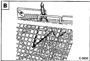
Remove the bolt and nut at the spring block. Remove the spring block (both sides) [C].
