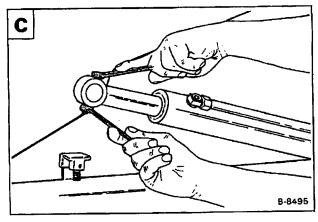
Remove the pins at the rod end of the lift cylinders (both sides)
