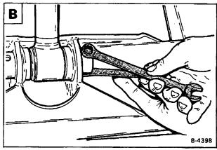
Remove the pivot pin at the rod end of the tilt cylinder C.
