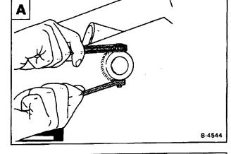
Use a punch and hammer and remove the pivot pins at the lift arms (both sides)  ${\bf B}$ .
