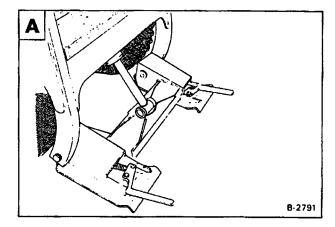
Remove the lock nut and bolt at the rod end of the tilt cylinder  $[\
