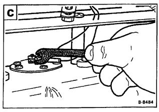
Disconnect the fuel hose at the shut-off valve D.
