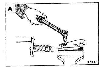
Remove the block from the wedge bolt B.
