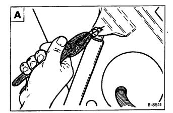
Remove the upper pivot pin for the gas cylinder (both sides) B.
