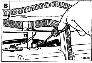
Disconnect the wires at the fuel sender C.
