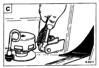
Remove the lower pivot pin (both sides) D.
