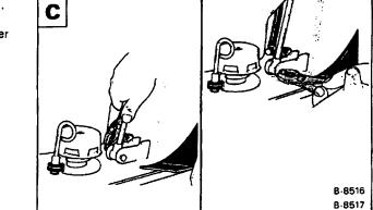
Remove the clip and lower pivot pin at the gas cylinder C.
