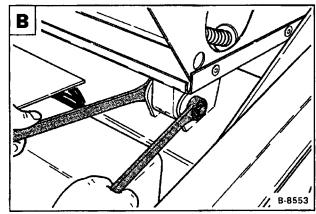
Use a punch to remove the pivot bolt (both sides) C.
