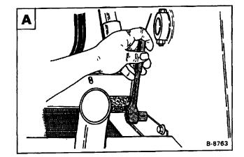
Remove the holddown bracket at the left side of the loader frame  $\ensuremath{\mathbb{B}}$ .
