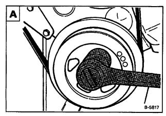
Installation: Tighten the bolt to 180 ft.-lbs. (245 Nm) torque B.
