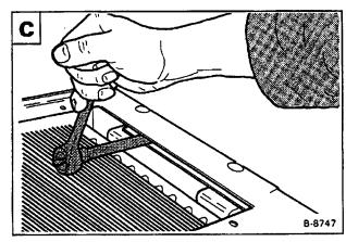
Remove the bolts at the left side bracket for the oil cooler  ${\color{red} {\bf D}}$ .
