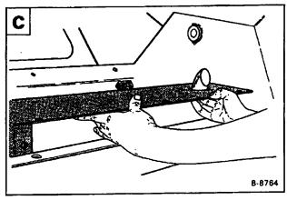
Remove the muffler from the loader D.
