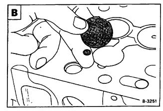
Make sure to check the height of the insert to the cylinder head as shown  $\ensuremath{\mathbb{C}}$ .
