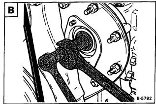
Remove the injection pump from the engine C.
