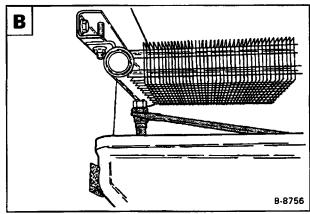
Remove the bolts at the right side bracket for the oil cooler C.
