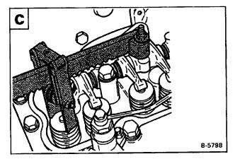
Install a dial indicator on the top of the valve stem D.
