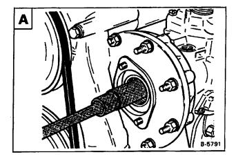
With the injection pump supported, loosen the pump gear using the special tool **B**.
