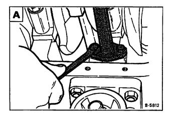
Loosen the locknut at the bolt which holds the oil pump in the block  $\ensuremath{\mathbb{B}}$ .
