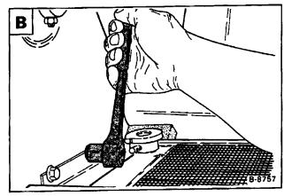
Lift the radiator up and remove it from the loader  ${\bf C}$  .
