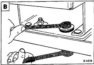
Remove the front engine mounting bolts, washers and nuts C.
