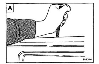
Use a punch and hammer and remove the rivet from the blower housing  $\ensuremath{\mathbb{B}}$ .
