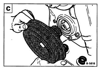
Remove the timing case cover from the engine D.
