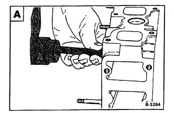
Position the new insert by putting the expansion washer in the correct position  $\ensuremath{\mathbb{B}}$ .
