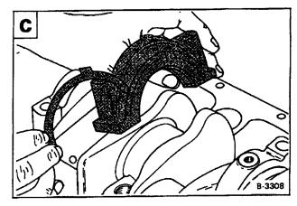
Remove the top half of the bearing and thrust washer by pushing on one side of the bearing and rotating the crankshaft  $\ \Box$ .
