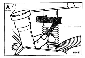
Remove the rear engine mounting bolts, washers and nuts B.
