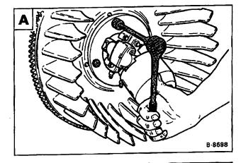
Remove the u-joint from the flywheel B.
