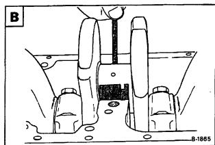
On the center main bearing, remove the cap and thrust washers from each side of the cap C.
