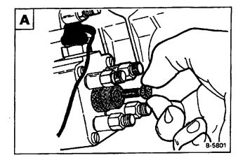
Install the timing tool and dial indicator so the plunger of the timing tool is against the pump plunger and dial indicator reads approximately 0.08" (2,0 mm) 8.
