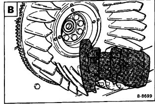
Remove the bolts from the flywheel [C].
