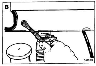
Remove the shield from the muffler C.
