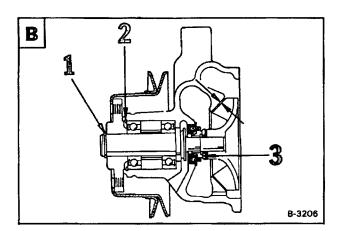
Press the impeller on the shaft. Check the clearance to make sure there is 0.015 - 0.030'' (0.38 - 0.76 mm) between the impeller and the housing  $\boxed{\textbf{C}}$ .
