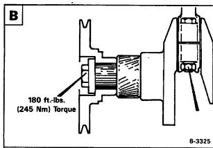
Remove the pulley from the crankshaft C.
