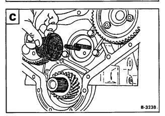
Check the idler gear and hub as the specifications shown D.
