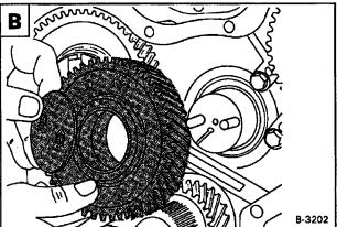
Remove the idler gear hub C.
