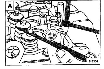
The correct clearance is 0.012" (0,30 mm) with the engine cold [8].
