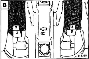
Remove the nuts and remove the bearing cap C.
