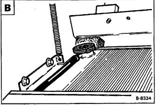
Open the coolant drain (Item 1) at the side of the engine block and drain the coolant into a container  $\boxed{\mathbf{C}}$ .
