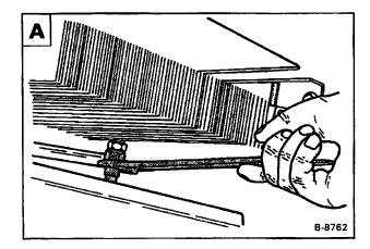
Disconnect the tubeline at the left side of the oil cooler B.
