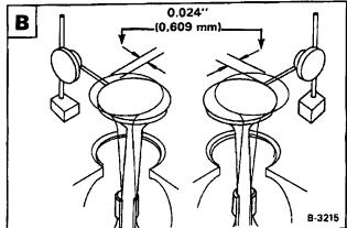
NOTE: Make sure to check the valve stem for wear before replacing the valve guide C.
