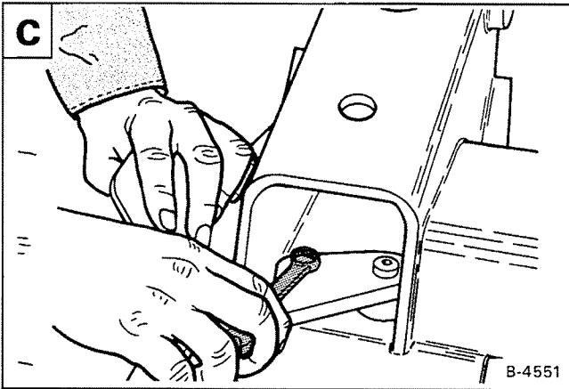
Using a punch and hammer, remove the Bob-Tach wedge and spring assembly from the frame **D**.
