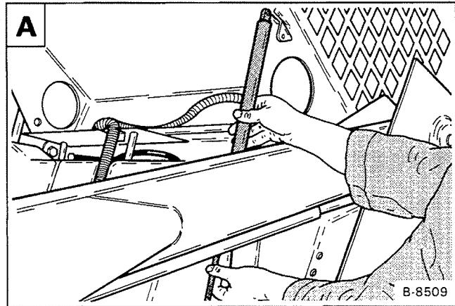
Remove the nuts from the pivot bolts **B**.
