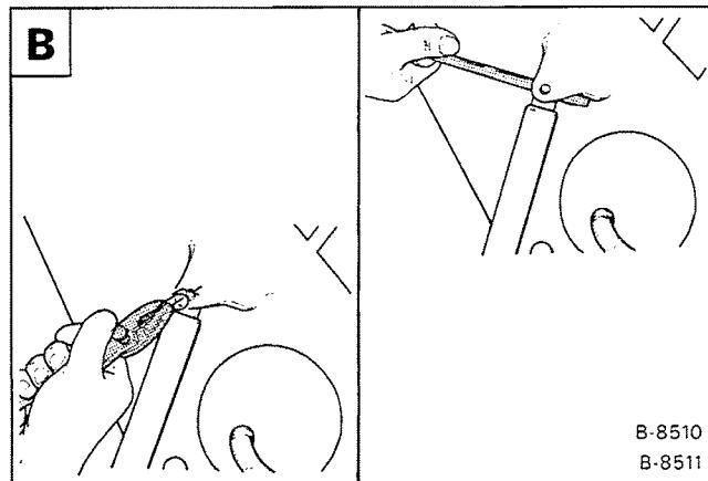
Remove the clip and lower pivot pin at the gas cylinder **C**.
