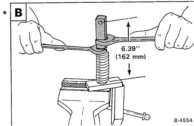
Remove the nut and the spring from the bolt **C**.
