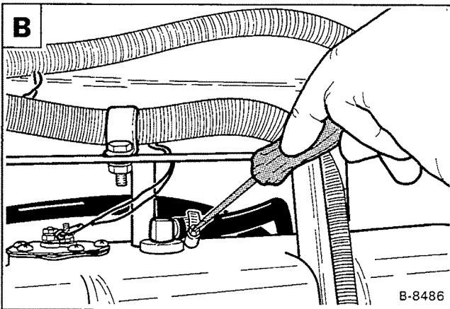
Disconnect the wires at the fuel sender **C**.
