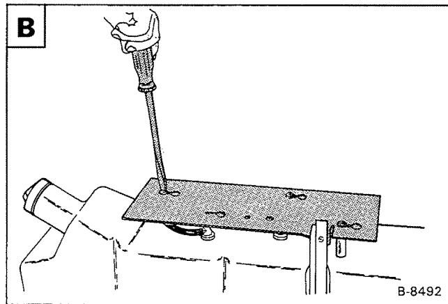
Remove the screws from the sender switch **C**.
