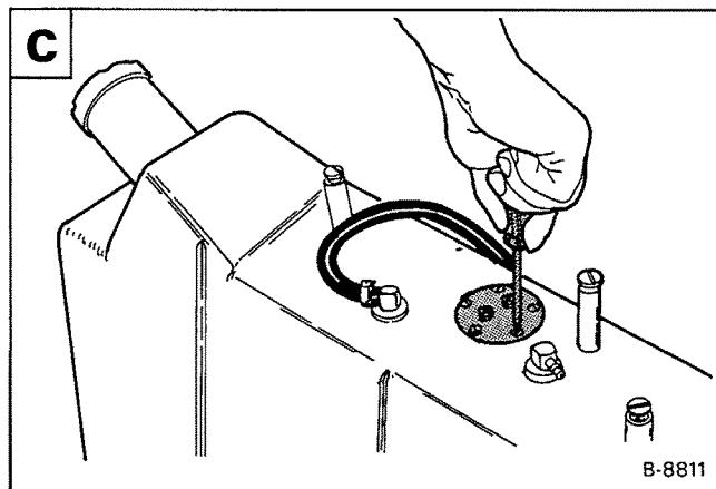
Remove the sender switch from the fuel tank **D**.
