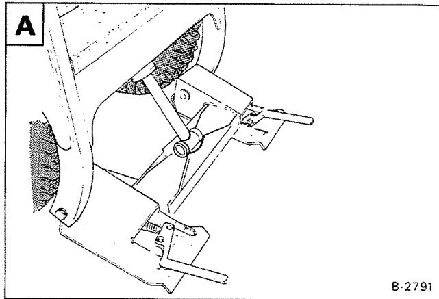
Remove the lock nut and bolt at the rod end of the tilt cylinder **B**.
