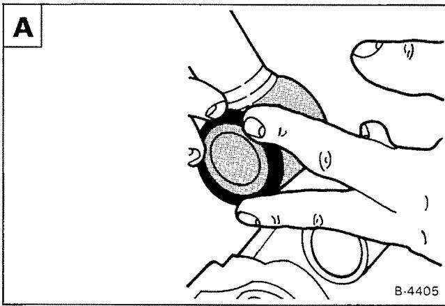
Put a piece of shim stock on each side of the seals **B**.
