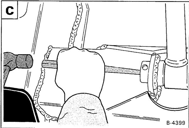
Loosen the bolt at the Bob-Tach pivot pin **D**. DO NOT remove the bolt.
