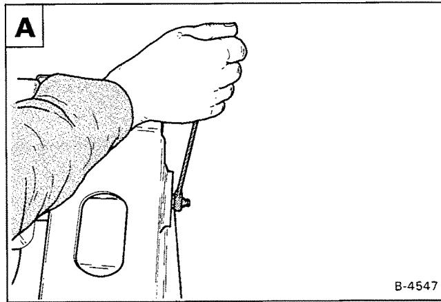
Hit the bolt to start the pivot pin into the Bob-Tach frame **B**.
