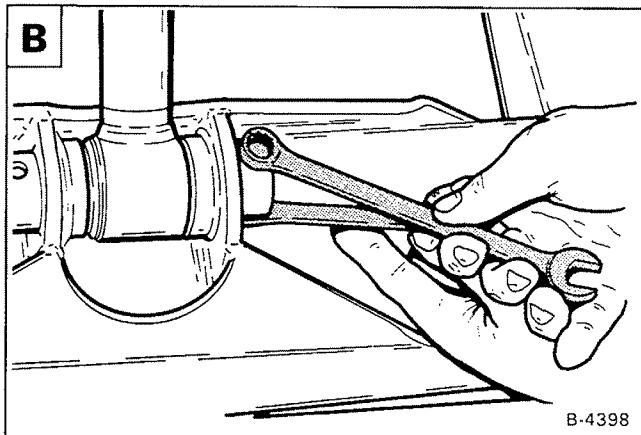
Remove the pivot pin at the rod end of the tilt cylinder **C**.
